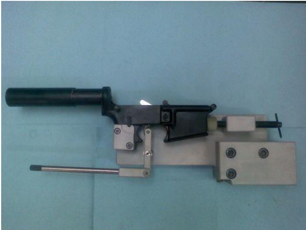
Figure 1. Test Firing Fixture
